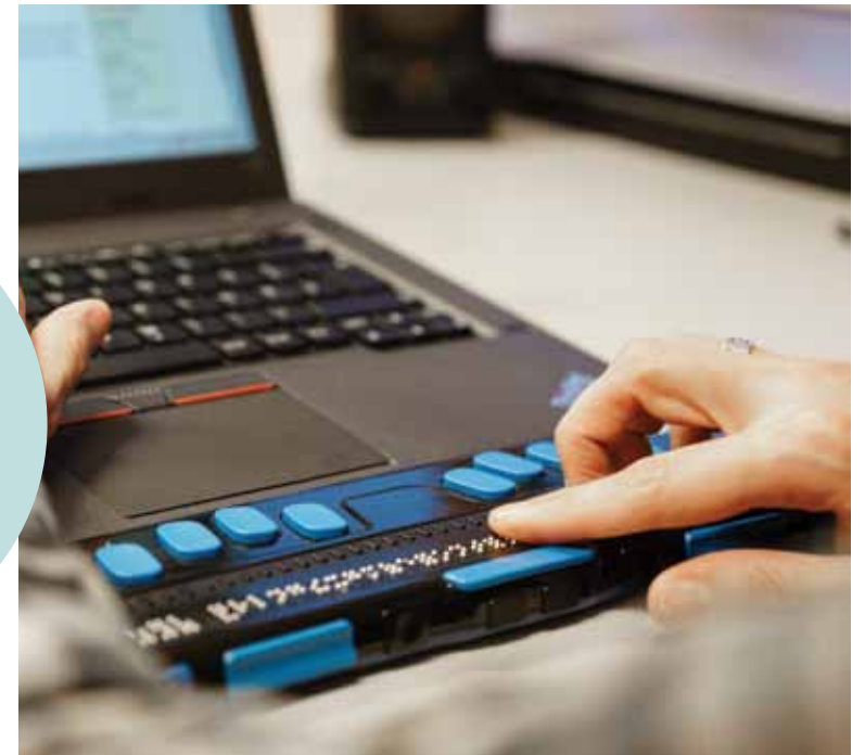
A laptop with a braille bar, which replaces the screen for blind people (photo: Michel Arriens, source: societypix.com)
