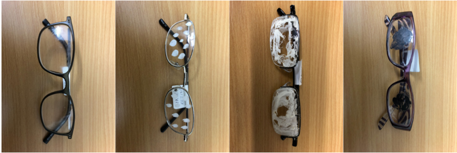
Fig. 2. Modified glasses to simulate conditions (Copyright: Helen Petrie).
