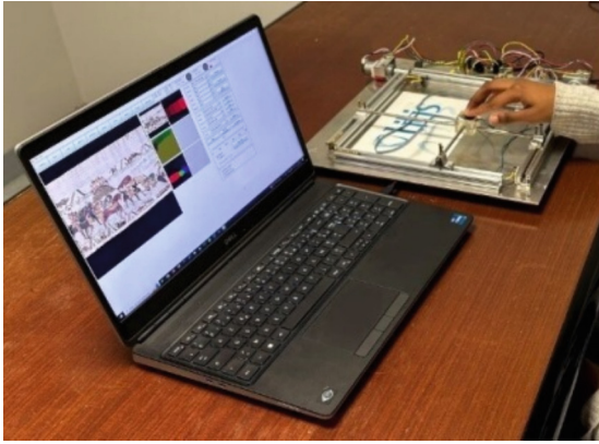
Fig. 1. F2T Force Feedback Tablet used to transmit a haptic impression of a virtual image. The joystick moves in 2D under the impulse of two motors on the horizontal and vertical axes.
